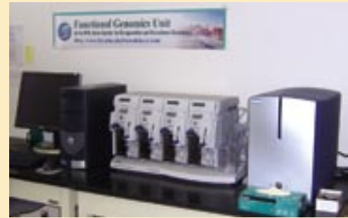
Affymetrix 3000 Workstation for processing and scanning GeneChips.
