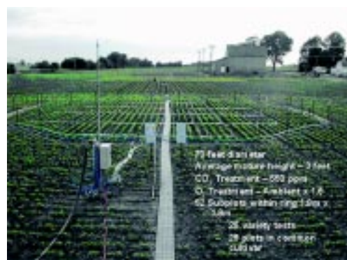
Figure 2. One of eight FACE rings that were operated in 2001. Within the ring soybean is grown from sowing to harvest at 550 ppm carbon dioxide, mimicking the level anticipated for the year 2050. The right side of this ring is planted to a single cultivar—that used throughout the field, the left side to 26 different lines. Currently corn is growing at the same location, also under elevated carbon dioxide.
