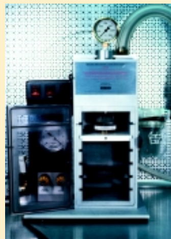
Plant Tissue Culture and Gene Transfer Facility. Bio-Rad Model PDS-1000/He Biolistic Gene Gun.
