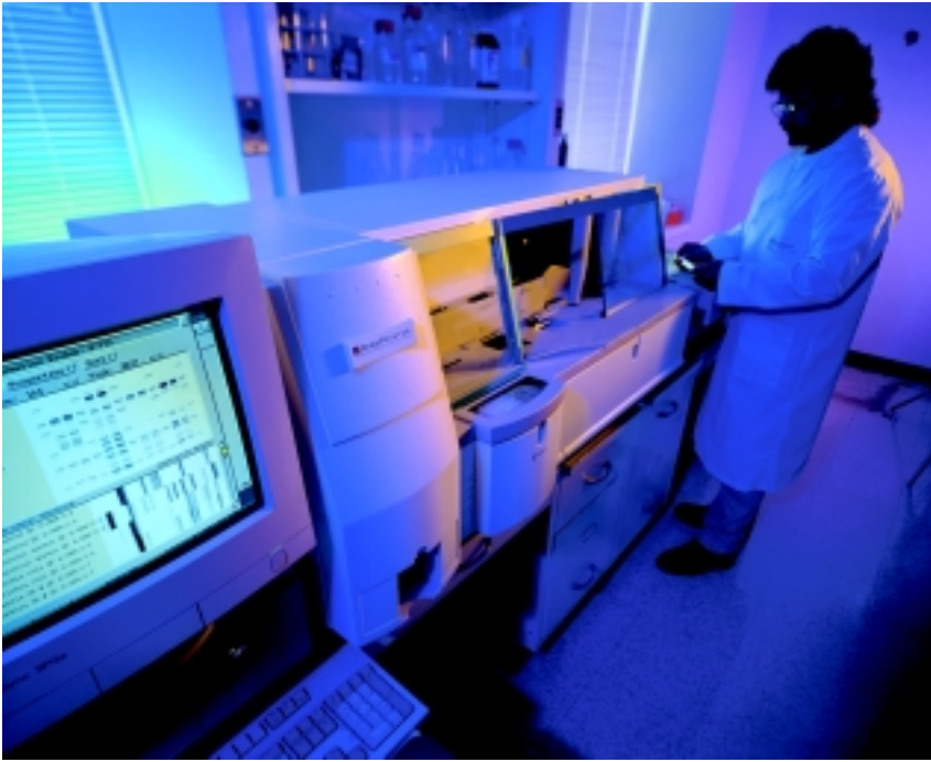
The RiboPrinter® microbial characterization system is the only fully automated instrument for fingerprinting the DNA of bacteria. It is made by Qualicon, a subsidiary of DuPont.
